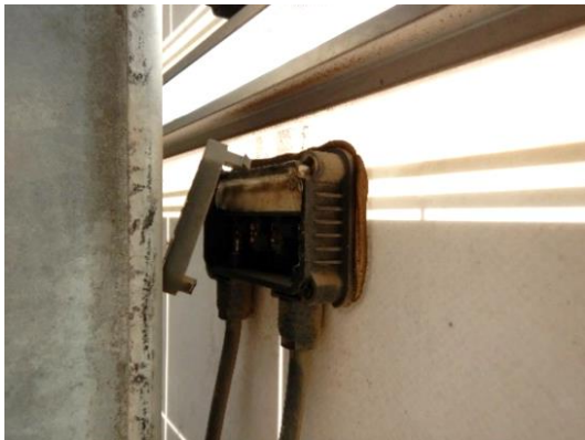
Figure 33: Broken J-Box lid
