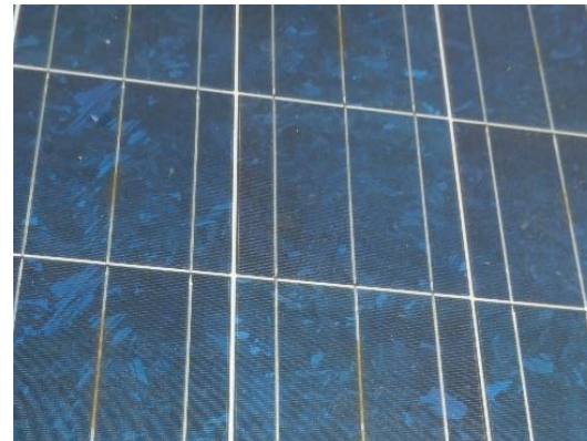
Figure 124: Broken and burned cells
