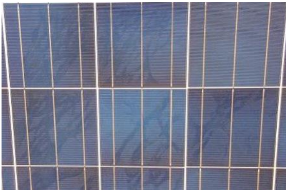
Figure 6: PV module showing snail trails [source: PI Berlin]
