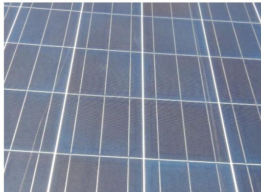
Figure 21: Cell "framing" or discoloration effect
