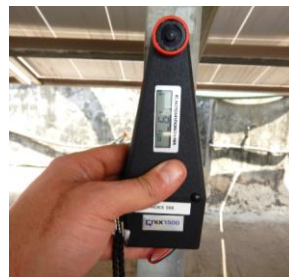
Figure 57: Coating thickness - galvanization
