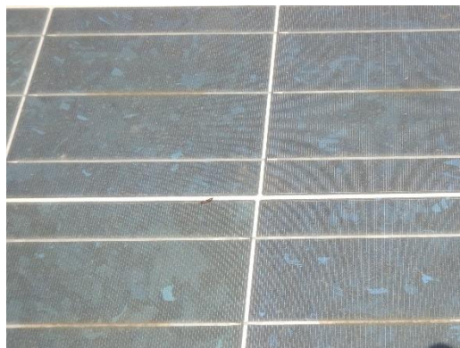
Figure 109: Corrosion in bus bars
