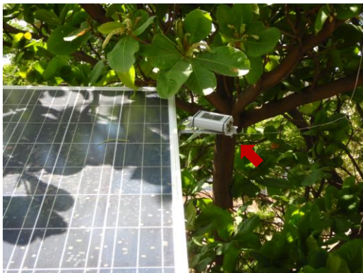
Figure 62: Shading and irradiation sensor situation
