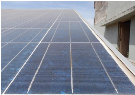
Figure 135: Modules with busbar corrosion
