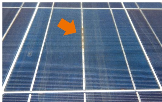
Figure 96: Modules with busbar corrosion
