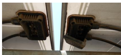
Figure 69: Modules with open or missing J-boxes
