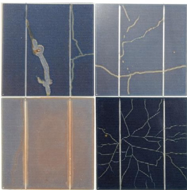
Figure 141: Examples of "cracks" found
