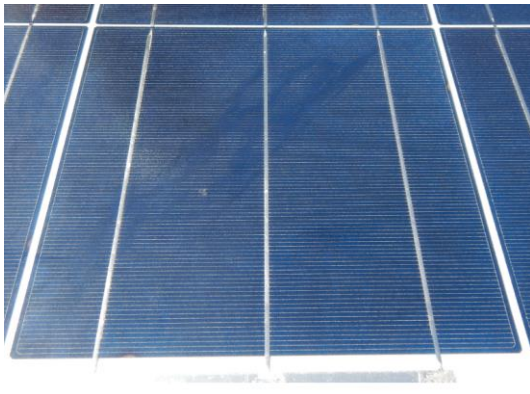
Figure 20: Snail trails (microcracks)
