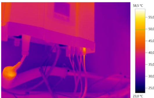
Figure 95: Hot connector at the inverter
