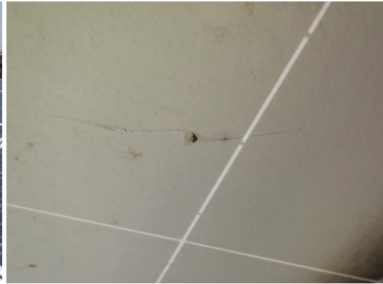
Figure 61: Module with scratch in the backsheet
