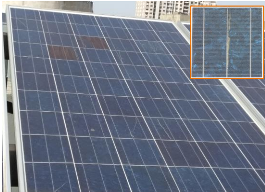
Figure 137: Advanced degradation cracks & hotspots
