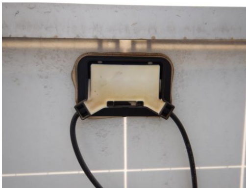
Figure 113: Junction box without lid
