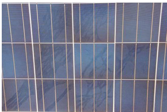
Figure 4: PV module showing snail trails [source: PI Berlin]
