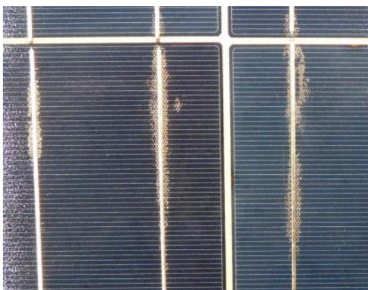
Figure 9: Delamination on the PV cells [source: PI Berlin]
