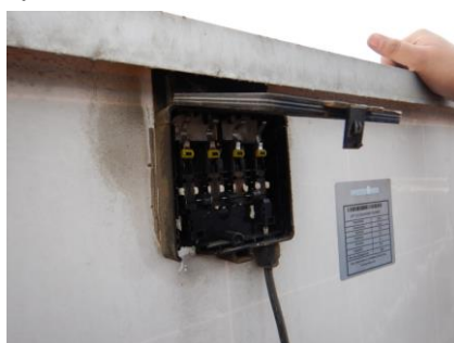
Figure 60: Loose junction box lid
