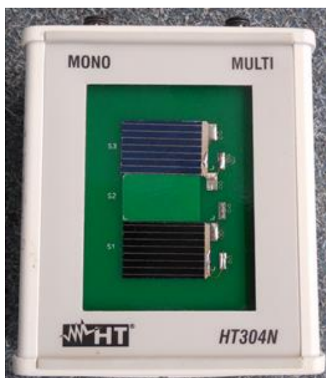
Figure 132: Duo reference cell [source: PI Berlin]
