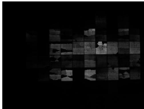
Figure 44: Cell cracks combined with PID
