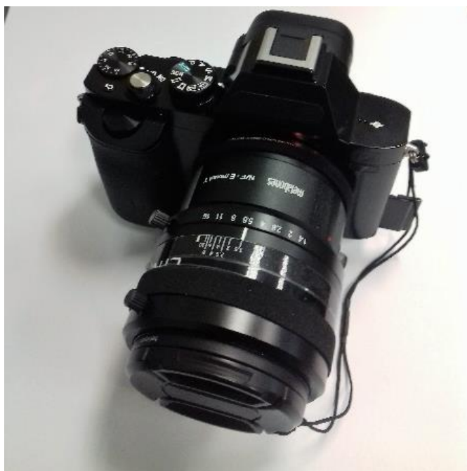
Figure 134: SONY ILCE-7S with CCD high pass edge filter [source: PI Berlin]
