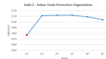
Figure 28: Irradiation increase vs. tilt angle
