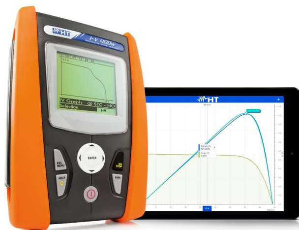
Figure 141: HT SOLAR-IV IV curve tracer [source: pv-engineering]
