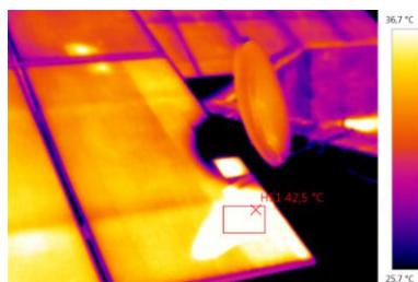
Figure 12: Hot spots caused by near shadings
