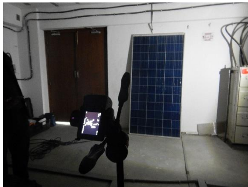
Figure 8: Electroluminescence (EL) set up
