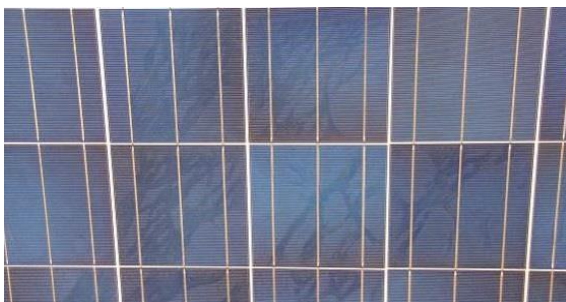
Figure 7: PV module showing snail trails [source: PI Berlin]
