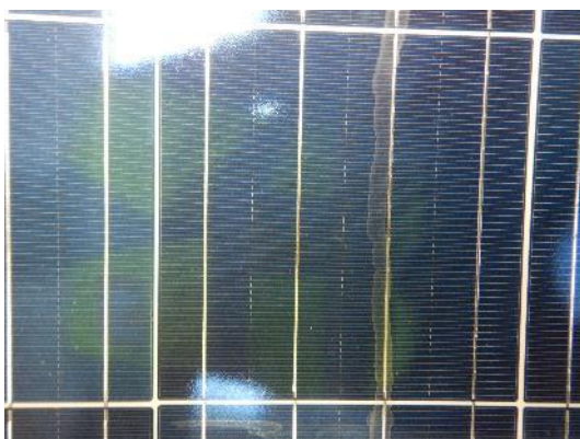
Figure 71: Soil on the module surface
