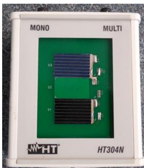
Figure 137: Duo reference cell [source: PI Berlin]
