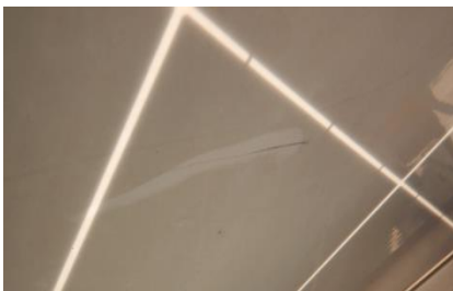
Figure 13: Scratch on the back sheet
