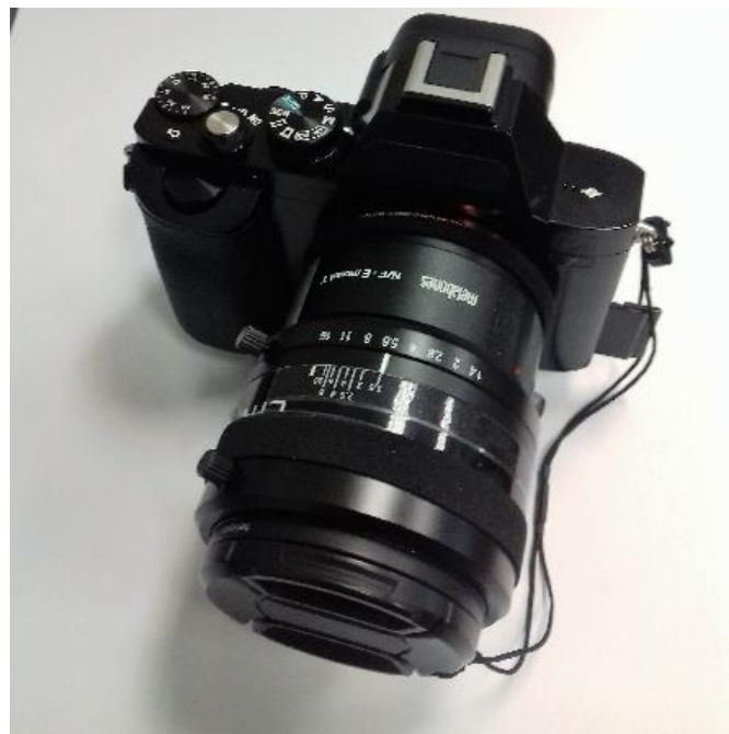
Figure 139: SONY ILCE-7S with CCD high pass edge filter [source: PI Berlin]
