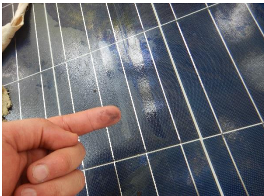
Figure 88: Exhaust residue on the module surface
