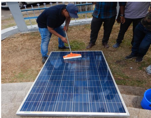
Figure 122: Module cleaning for IV curve test
