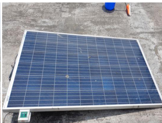
Figure 133: Bird drops on module glass
