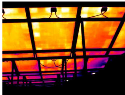
Figure 55: IR image of PID modules
