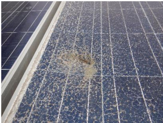
Figure 36: Module glass breakage
