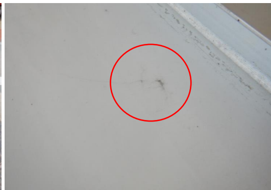
Figure 121: Mechanical damages in module BS
